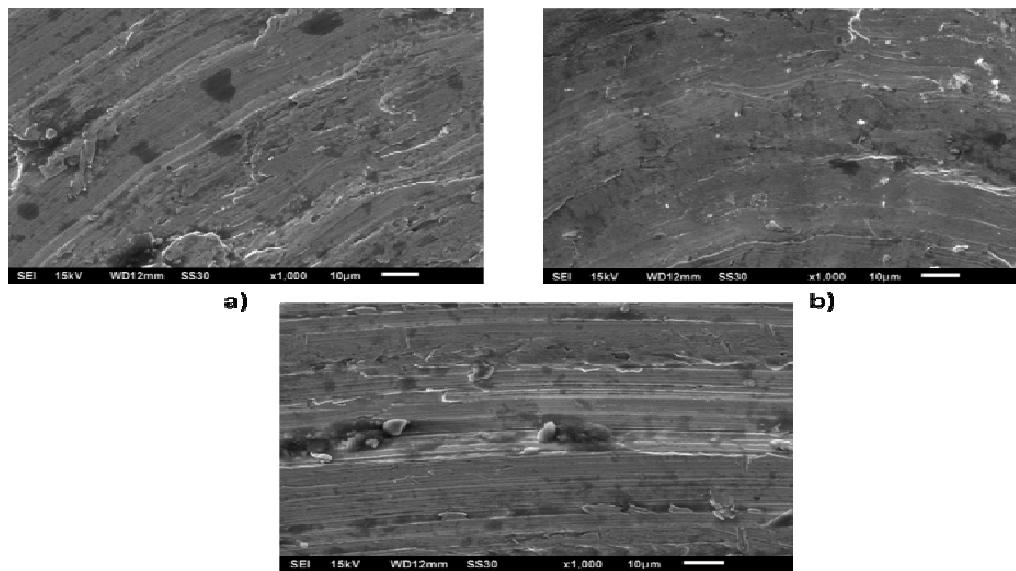
**Fig. 2.** SEM images (before machining) of three electrodes, a) Steel-304, b) Brass and c) Copper.
