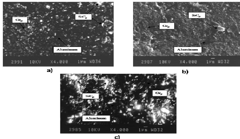
**Fig.1.** SEM images of three fabricated composites, a) Al MMC-1 (SiCp10% and Grp3%), b) Al MMC-2 (SiCp15% and Grp5%) and c) Al MMC-3 (SiCp20% and Grp8%).
